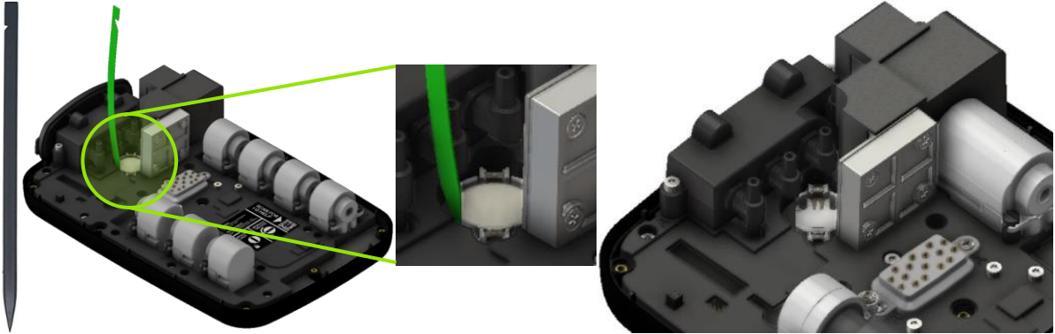
Figure 11 – Coin Cell Removed
