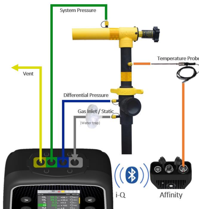
Figure 4 - i-Q Connection to QED Wellhead
