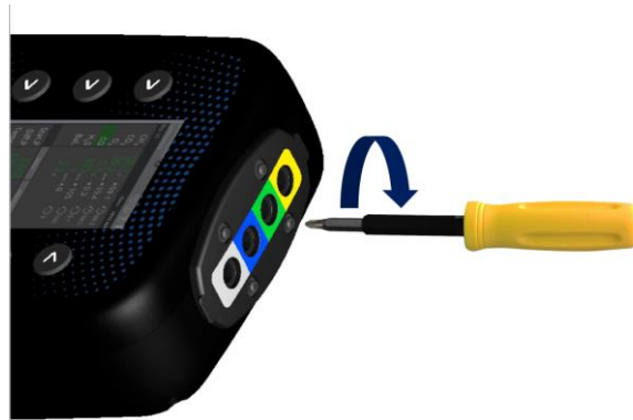
Figure 15 – Inlet Port Plate Fitting
