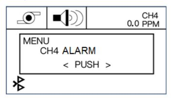
When the measured gas concentration has exceeded the alarm threshold, the red LED's will illuminate and the acoustic alarm will sound.
