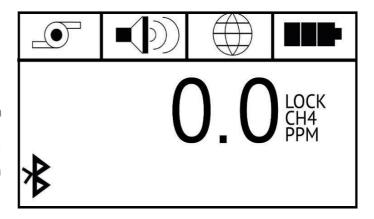
When the concentration drops back below 0.1%VOL, the blue LED bumper remains ON to indicate that the METREX remains in %VOL mode. To return to ppm mode, press the down arrow/0 key when the concentration is less than 1.0%.
