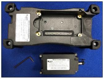
Battery pack removed from instrument
