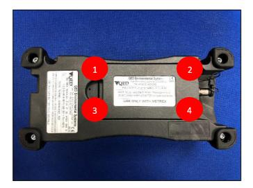
Unscrew the four battery screws
