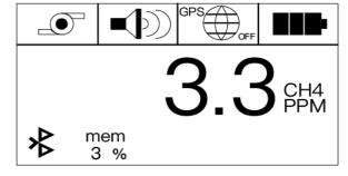
While a menu is active, the gas value is displayed in the upper right corner of the display [D].
